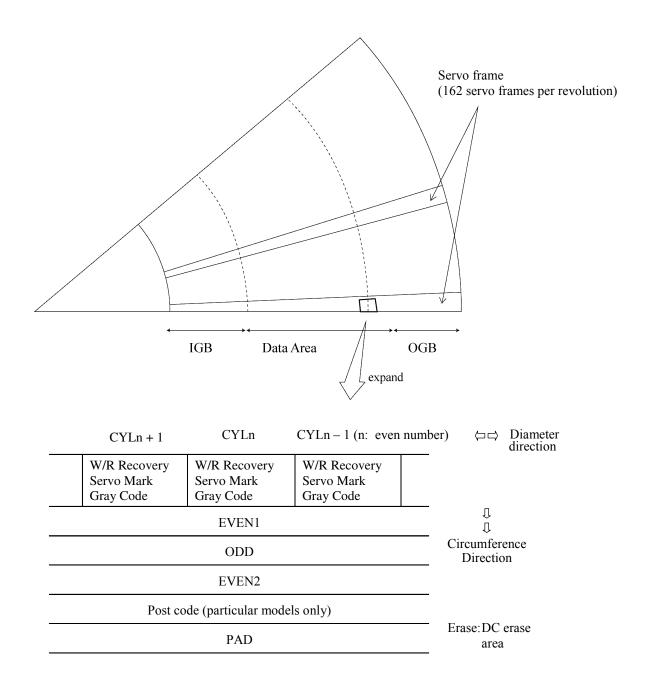
Figure 4.7 Physical sector servo configuration on disk surface
